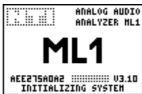
Fig 5.1 Start Up Screen Loading Default Setup
