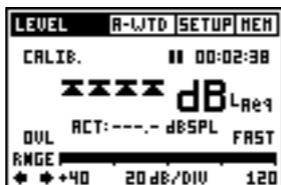
Fig 3.4 SPL Panel with Overload
