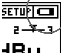
Fig 2.6 Low Battery Indicator
