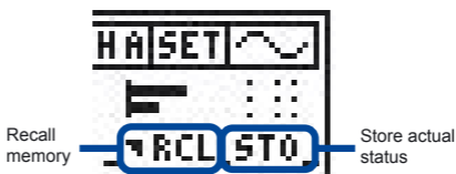
Fig 5-08, Channel status memory field
